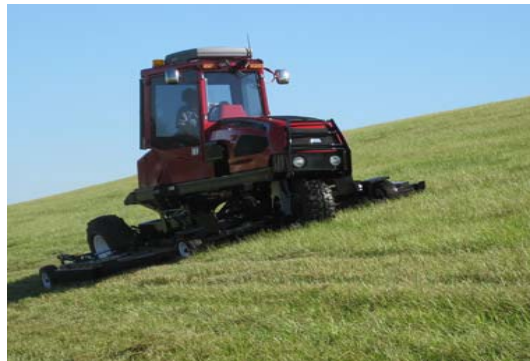
Figure AX2.4: Maintaining Grass on Embankment
